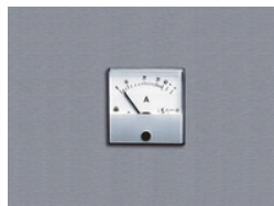
Ammeter - blade load indicator
